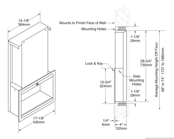
Rough Wall Opening: 15-5/8" (397mm) Wide 29-1/4" (743mm) High 4" (102mm) minimum recessed depth
