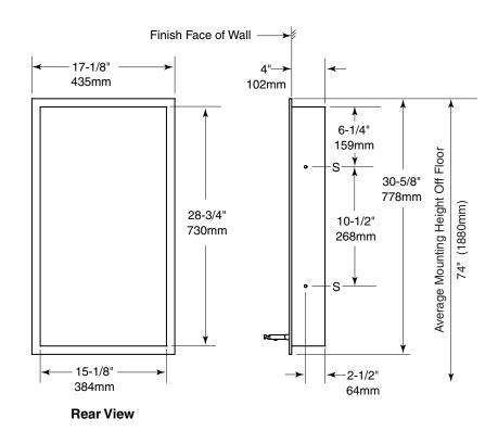
Rough Wall Opening: 15-5/8" (397mm) Wide 29-1/8" (740mm) High 4" (102mm) minimum recessed depth
