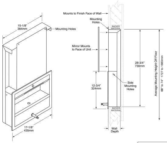
Rough Wall Opening 15-5/8" (397mm) wide 29-1/8" (740mm) high 6" (152mm) minimum recessed depth
