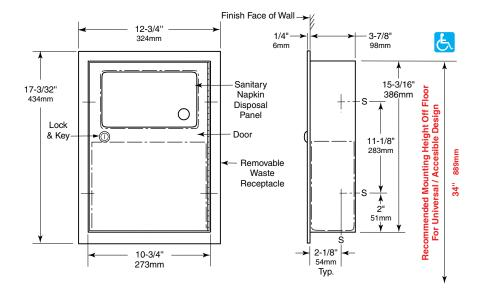
Rough Wall Opening 11" (279mm) wide 15-7/16" (392mm) high 3-15/16" 100mm) minimum recessed depth
