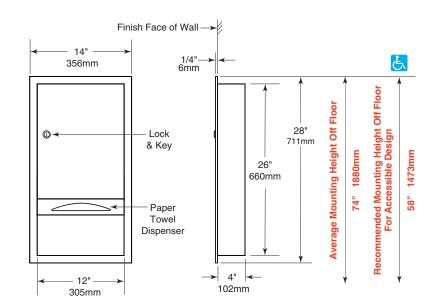
Rough Wall Opening 12-1/2" (318mm) wide 26-1/2" (673mm) high 4" (102mm) minimum recessed depth
