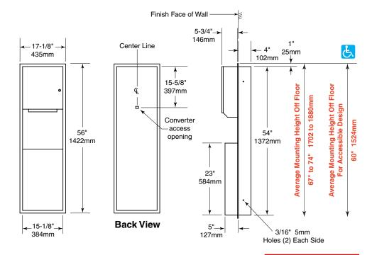
Rough Wall Opening 15-3/4" (400mm) Wide 54-3/4" (1391mm) High 4" (102mm) minimum recessed depth
