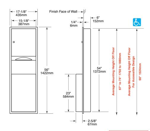
Rough Wall Opening 15-3/4" (400mm) wide 54-3/4" (1390mm) high 6" (152mm) minimum recessed depth
