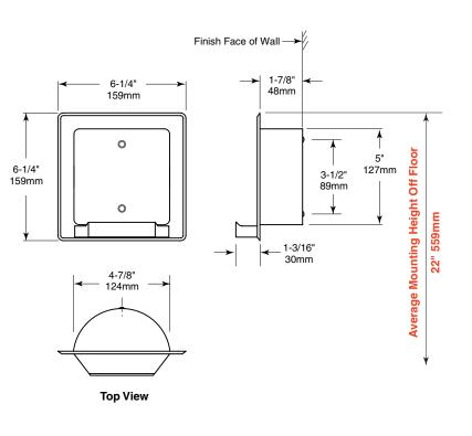
Rough Wall Opening: 5-1/4" (133mm) Wide 5-1/4" (133mm) High 2" (51mm) minimum recessed depth
